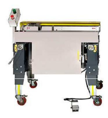
The operator opens the flat case and places it into the erector. The machine folds the bottom flaps ready for packing. After packing, the operator presses the foot-switch or push-button. The machine automatically pushes the case into a case sealer, saving time and labour costs.
