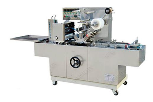
Camphor block cellophane wrapping machine is a fully automatic cellophane packaging machine, mainly used for packing bulk poker, cigarette box, perfume box, cosmetic box, VCD/DVD tape, medicine box, note paper etc. It can pack with tear type.
