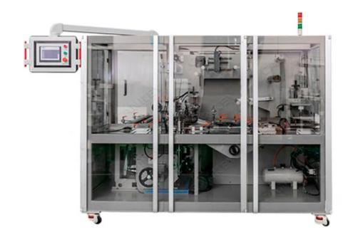
This tea box cellophane overwrapping machine adopts multi-function digital display frequency conversion stepless speed regulation, PLC programming control technology, automatic box feeding and automatic counting, which is perfect for wrapping tea box, medicine box, perfume box, cigarette cartons, cosmetic box etc.
