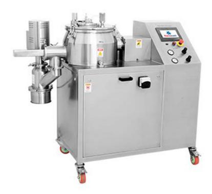
The lab-scale rapid mixer is mainly used in R&D or F&D facilities for the wet mixing of Small batches. Basically, it consists of a Bowl, Impeller & Chopper assembly. The high shear wet granulation process is extensively used in the pharmaceutical industry to transform fine heterogeneous powders into a homogeneous blend of granules with bigger size and density to improve flow and compatibility for tableting operation.
