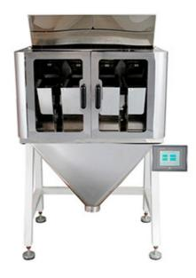
It's suitable for weighing slice, roll or regular shape products such as sugar, salt, seed, rice, sesame, glutamate, milk powder, coffee and seasoning powder, etc.
