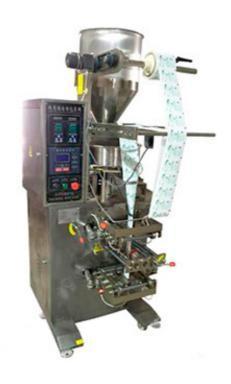
Automatic Sugar Sachet Packaging Machine adopts correcting system controlled by microcomputer, owing to a response signal is handle and pass through microcomputer. It can accomplish whole set to synchronization, sack length, position fixing, voluntarily follow the tracks of light-mark and voluntarily diagnose trouble and show to screen.
