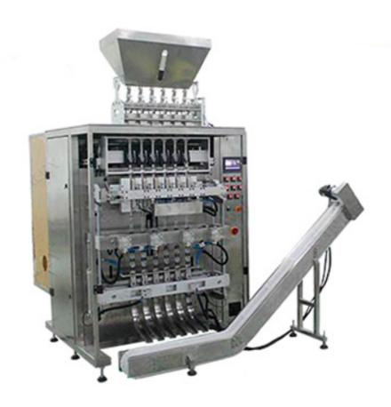
Multi lanes sugar sachet filling machine is a self-developed packaging device based on advanced foreign similar models. It is suitable for loose, non-sticky and certain flow able granular materials in pharmaceutical, food, daily chemical and other industries.
