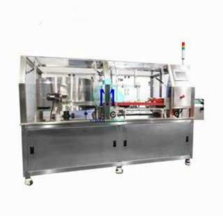
The Bottle Unscrambler Machine is used to automatically orient and feed containers into the production line. It can unscramble plastic, metal, and other non-fragile containers.
