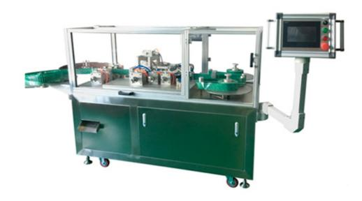
SJ-7ZK Full-automatic Suppository Production Line is suitable for the production of special shape such as bullet head, torpedo shape bill, to meet the production of your suppository.
