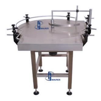
We adopt frequency stepless governor for a rotary motion, making all the bottles enter into converyer belt sequentially under the rotary tangential force to reach. The target of labor, boost production efficiency. This machine can be used when it is electrified. Easy operating, it can be widely used for glass bottles, plastic bottles and polyester bottles for pharmaceutical, agrochemical, food, chemical etc. It is a good choice for small, medium, large factory.
