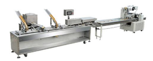
A biscuit sandwiching machine is a kind of packaging equipment which is widely used in the packing of biscuits, cookies, chips and other snacks. The machine is an ideal piece of equipment for making 2 or 3-layer biscuits. It can produce high-quality biscuits with different shapes and thicknesses.
