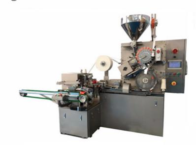
DXDC8IV model tea bag packing machine is new developed, with thermal sealing and multifunctions, it's the necessary for bag-type drinking's automatic packing.
