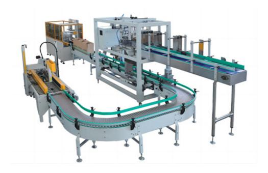
Suitable for various shapes of bottle carton packing, automatic bottle carton packing machines widely use in round, square, triangle bottles etc.
