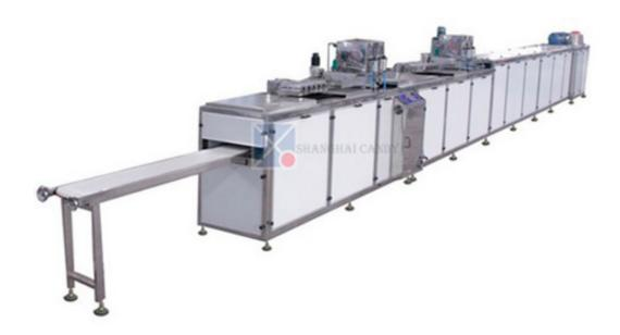
This machine services as advanced chocolate pour-forming equipment that integrates mechanical control and electric control all in one. Full automatic work program is applied throughout the flow of production, including mould drying, filling, vibration, cooling, demolding and conveyance. This machine can produce pure chocolate, chocolate with filling, two-color chocolate and chocolate with granule mixed. The products enjoy attractive appearance and smooth surface.
