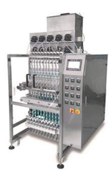
Multi Lane Liquid Packing Machine automatically finishes the process of filling, metering, bag forming, air exhaust, sealing, packing, and date printing.
