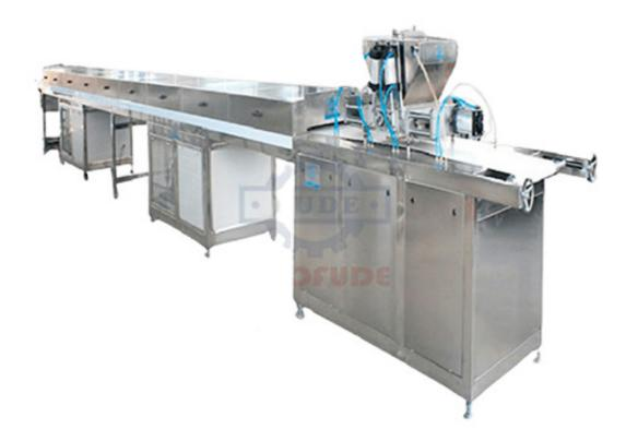
Chocolate Chip Machine is for depositing chocolate chips. The chocolate drops/chips can be poured on the conveyor belt directly, and the weight of each drop can also be adjustable.
