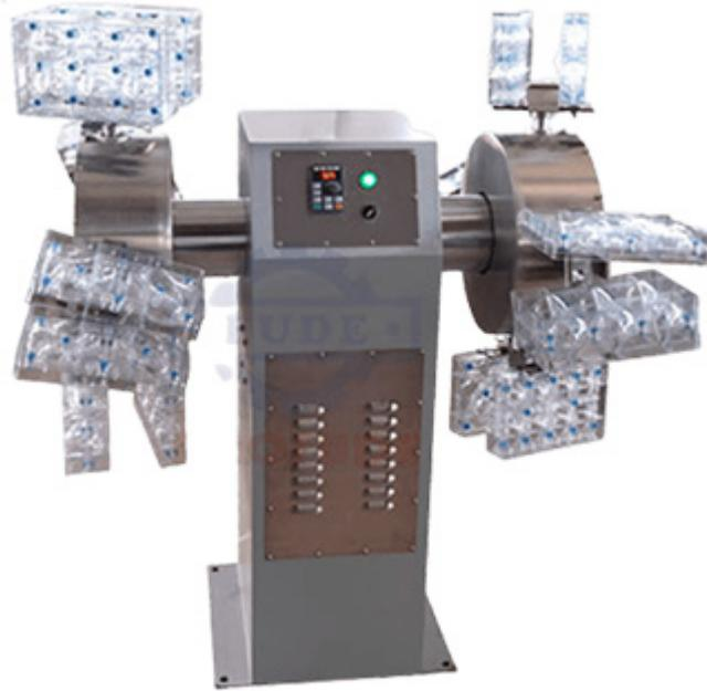
CKX-4 Hollow Chocolate Spinning Machine is designed to produce hollow chocolate products with special hollow PC molds. The machine uses the theory of eccentricity by revolution and rotation techniques to produce hollow chocolate products. These lovely, novel, solid shapes of hollow chocolate products present high-quality artwork and a dense economy attachment.
