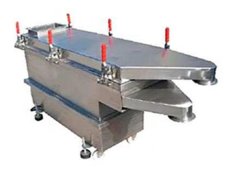
The Machine consists of screen box at material inlet and outlet, vibrator and shock absorber. There are 4-6 sets of flexible rubber shock absorber connected between base and screen box in up-down order. Centrifugal force is generated upon starting the machine. Control shock absorber against amplitude eccentric device correspondingly for best performance and material screening process in throwing vibration and loose.
