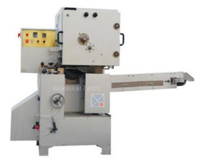
The line is composed of dissolving tank, storage tank, vacuum cooker, cooling table, batch roller, rope sizer, forming machine, transporting belt, cooling tunnel etc. The forming dies for hard candies are in a clamping style which is an ideal device for producing different shapes of hard candies and soft candies, small wastage and high production efficiency. The whole line is manufactured as per GMP standard in accordance with the requirement of GMP Food Industry.
