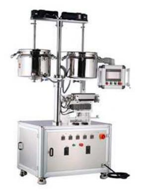
Automatic Lipstick Filling Machine has the advantages of easy to clean, high efficiency and application widely. It is suitable for filling a lipstick, lip balm, foundation cream, pearl cream, eye shadow and other liquid or paste materials.
