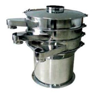
The machine consist of hopper, vibrating chamber, coupler and motor. There are eccentric wheel, rubber software, main shaft and shaft-bearing in the vibration chamber. The adjustable eccentric hammer is driven to the center line through the motor, cause centrifugal force under the state of unbalance and so that the materials form regular eddy. The amplitude of the hammer may be adjusted according to the property of material and the mesh screen.
