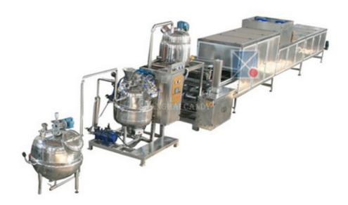
Toffee depositing line is the most advanced equipment for continuous making toffee caramel candy. It gathered machinery and electric all in one, using the silicone moulds automatically depositing and with tracking transmission demolding system. It can make pure toffee and center filled toffee. This line consists of jacketed dissolving cooker, transfer pump, pre-heating tank, special toffee cooker, depositor, cooling tunnel, etc.
