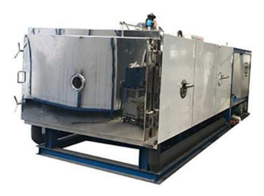
FD-30L is an commercial and industrial Freeze Dryer for process material bulk production, meet FDA and cGMP request, could use for bio-pharmaceutical, biological, chemical, solvent, tissue bank design and produce under GMP, Available shelf area 29.8sq.m,11 shelves, 99 trays and ice capacity 400L in 24hrs, Final vacuum <1Pa.
