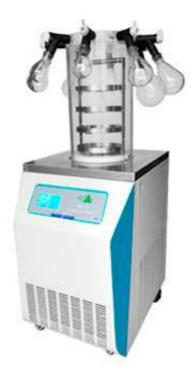
Dryer is widely used in medicine, pharmacy, biology research, chemical industry and food production, etc. After the freeze drying process, a long term preservation is much easier. They can be restored to the original state and mantain their chemical and biological characteristics after being watered. This model is suitable for experiment in laboratory and small amount production, and it can meet the regular freeze dying requirements of the most laboratories.
