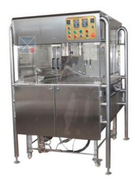
The enrobing machine is to coat chocolate on various food such as biscuit, wafers, egg-rolls, cake pie and snacks, etc. It mainly consists of chocolate feeding tank, enrobe head, cooling tunnel.
