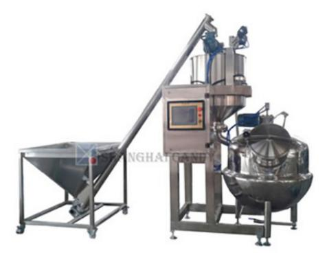
This machine offers automatic weighing, dissolving, mixing of raw material with inline transport to one or more production lines.
