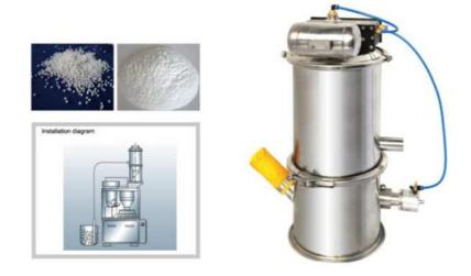
The QVC automatic vacuum feeding machine utilizes compressed air to realize material conveying. Requiring no mechanical type vacuum pump, the compressed air passes through the vacuum generator of the vacuum feeder, thus high vacuum environment is created. Thanks to the high vacuum, the material layering is fully avoided, ensuring the uniform mixing of the material.
