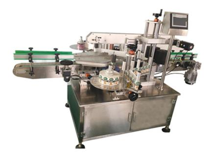
DTB-100 vertical type round bottle adhesive labeling machine is suitable for pharmacy, chemical industry and foodstuff etc round container labeling. The labeling process is fully automatic. Operation is easy, production speed is fast. Labeling position is accurate.
