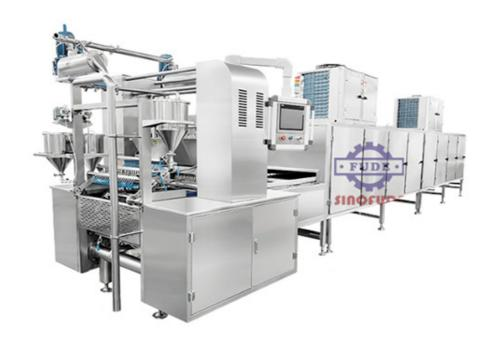
This is an automatic gummy candy production line designed for gummy candy manufacturers. It is a high-speed, efficient and reliable machine that can produce up to 80 kg of gummy candies per hour. With this machine, you can produce various gummy candies in different shapes and sizes. It is easy to operate and requires minimal maintenance. So if you are looking for a high-quality, automated gummy candy production line, the CLM80 is a perfect choice.
