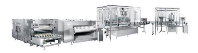
Glass bottle IV solution production line is a high-tech equipment that can automatically complete the processes of glass bottle cleaning, filling, stoppering, capping etc. for IV solution of 50ml-500ml. It is suitable for the production of various kinds of liquids, such as glucose, antibiotic, amino acid, fat emulsion, nutrient solution and biological agents etc.
