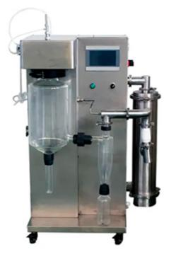
The LPG Series Laboratory Spray Dryer operates based on the principle of atomization and rapid evaporation. It takes a liquid feed material and transforms it into a fine powder or granular form through a two-step process. The liquid feed material is atomized into tiny droplets using a specially designed atomization system. This creates a large surface area and enhances the contact between the liquid and the hot drying gas.
