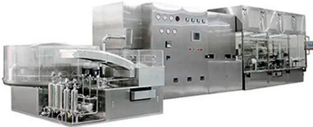
The Ampoule SVP Injectable Liquid Filling Production Line includes Ultrasonic washing machine, Sterilizing tunnel, Ampoule filling and sealing machine. Its divided into washing zone, sterilizing zone, filling and sealing zone. This compact line can work together as well as independently. Compared with other manufacturers, our equipment has unique features, including overall dimension smaller, higher automation & stability, lower fault rate and maintenance cost, and etc.
