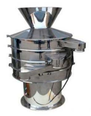
Main application This Sifting Machine is applied for the sorting of the granule size of dry power material in the trades medicine, chemical and foodstuff etc. Structural Characteristics The Sieving Machine is composed of the vertical vibration motor a sieve bottom a mesh frame sieve room rubber vibrating bowl and all fastening pieces, etc. This Sifter Machine can be operated for the sorting purpose either in single sieve or multi-sieves with a compact structure easy operating.
