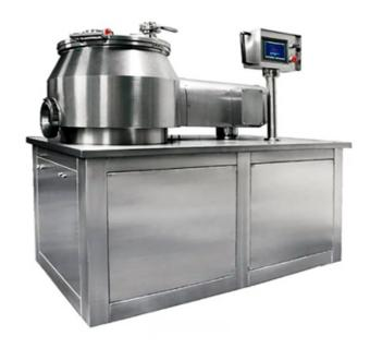
The High speed GHL series wet type mixing granulator is an advanced wet granulator which can effectively mix the target materials to turn out fine quality wet granules, and is widely applied by the trades of pharmacy, foodstuff, chemical, powder metallurgy, and dyeing etc.
