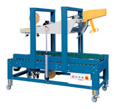
The CHS-6605A has automatic random flaps folding and top and bottom sealing. The machine comes with fully automatic adjustment on height and width for various sizes cartons. According to customer requirements 2' or 3' tapping heads can be included. Carton sealers have been designed and manufactured according to CE Standards.
