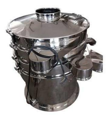
ZS vibrating Sifting Machine is composed of sieve box, vibration source and shock absorber. Vibration frame and screen box connected with rubber shock absorber fixed up and down, the production of centrifugal force, by the shock absorber control floating amplitude, so that the material has a downward shock throwing and downward stratified filtering process, so as to achieve a better classification screening effect.
