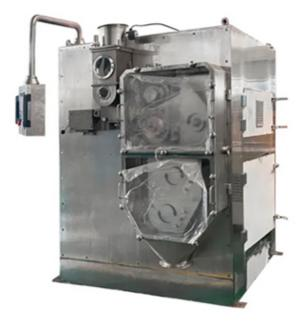
Dry granulator is the use of dry roller technology. In the process, fine powders are compacted mechanically into denser flakes. These flakes are subsequently crushed into finer granules. The grain size of the granules is determined by the suitable choice of the screen mesh size, especially the heat sensitive, humidity sensitive material granulation, widely used in pharmaceutical, food, chemical, powder metallurgy, printing and dyeing industries.
