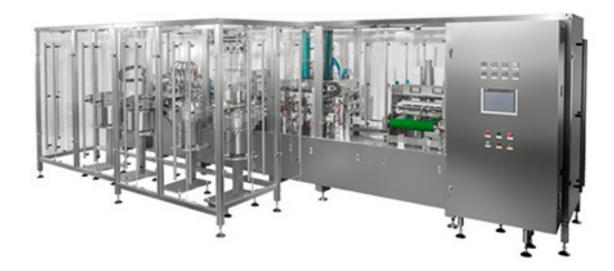
IVEN Pharmatech Engineering proudly presents its cutting-edge Non-PVC soft bag IV solution production line, incorporating the latest advancements in technology. This sophisticated system seamlessly executes film feeding, printing, bag manufacturing, filling, and sealing within a single, integrated machine.
