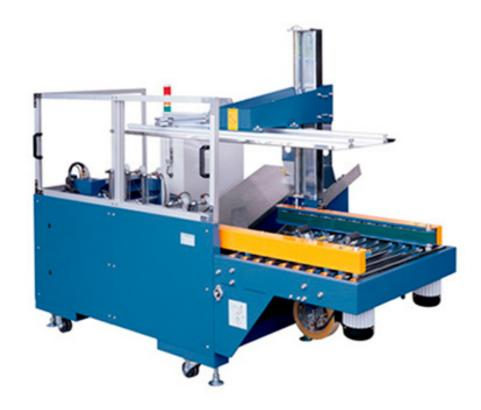
Our CHS-6701 is a vertical type Automatic Carton Erector. This Automatic Carton Erector Machine – Box Erector Machine is useful in bulk productivity in short duration, erecting cases of various sizes into different shapes and seal the bottom of the box with tape/hot glue. Carton erecting machine is very much useful and in high demand for auto packaging line.
