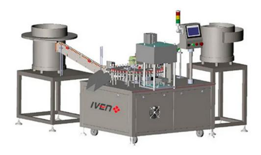
Our Virus Sampling Tube Assembling Line is mainly used for filling transport medium into virus sampling tubes. It with high degree of automation, high production efficiency, and have a good process control and quality control.
