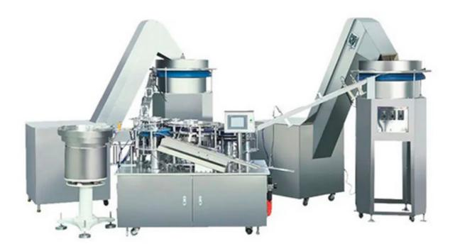
Our Syringe Assembling Machine is used for assembling syringe automatically. It can produce all kinds of syringes, including luer slip type, luer lock type, etc.
