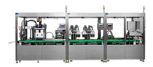
The blood collection tube production line includes tube loading, Chemical dosing, drying, stoppering & capping, vacuuming, tray loading, etc. Easy & safe operation with individual PLC &HMI control, only need 2-3 workers can run the whole line well. Compared with other manufacturers, our equipment has unique features, including overall dimension smaller, higher automation & stability, lower fault rate and maintenance cost, and etc.
