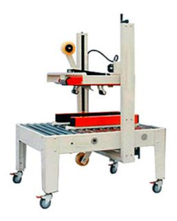
SP 102TU (Heavy Duty) Carton Sealer fits for continuous sealing of bigger cartons in the different size, which can be operated alone and also can be equipped into production line.
