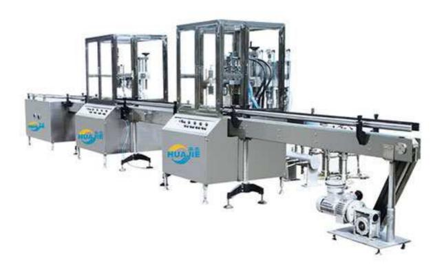
The whole machine is controlled by pneumatic and can be controlled separately. The main pneumatic control part are imported from Italy. No can, no material out. Equipped with one sealing head, 3 gas filling heads, 2 pressure pumps and 1 pc air storing tank. The whole machine is controlled by pneumatic, the main control element is imported from Japan or Italy.
