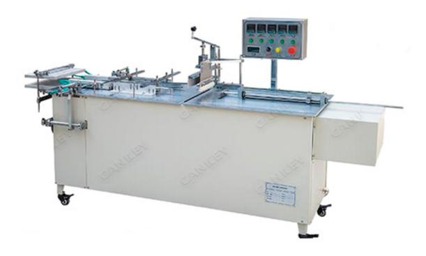
Semi-automatic Cosmetic Box Cellophane Wrapping Machine is for conveying, wrapping and counting. Easy to change moulds for wrapping products with different size. This semi-automatic 3d packing machine is widely used for test paper, cosmetics, medicines, food, health care supplies, audio and video products, stationery, daily necessities, packing effect is the same to cigarette packing.
